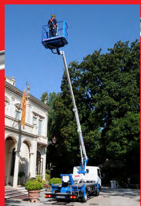
POSSIBILITY OF WORKING WITHOUT STABILISERS IN A REAR AREA
